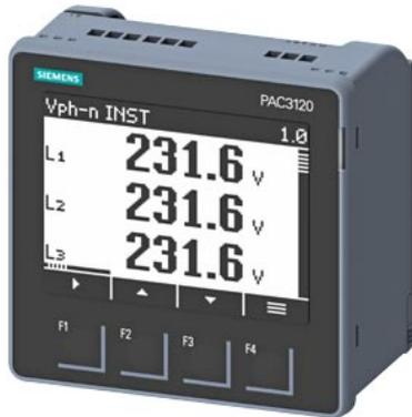
SENTRON PAC3120 LCD 96X96 mm Power Monitoring Device Control panel instrument for electrical values protocol: Modbus RTU with graphics display U rated input: 690/400V 45-65Hz IE rated input: X/1A oder X/5A AC Power supply: 24 ... 60 V -20/+10 % DC screw connections
